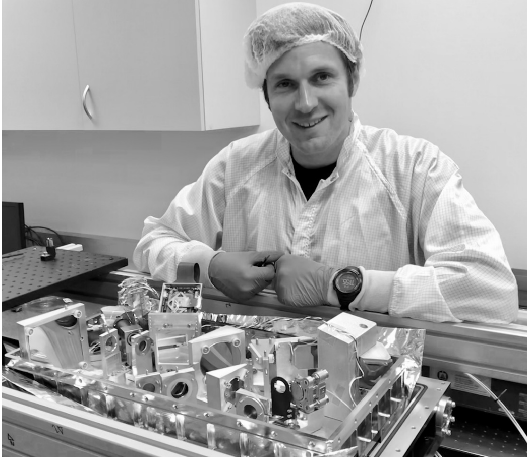
PARVI is incredibly compact for an R- 110,000 spectrograph
